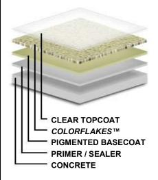
For best results, 10-15 mils of clear top-coating is recommended to fully encapsulate ColorFlakes™ and provide a durable wearing surface.
